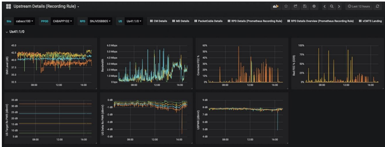
Figure 2 - Grafana dashboard used for network monitoring
