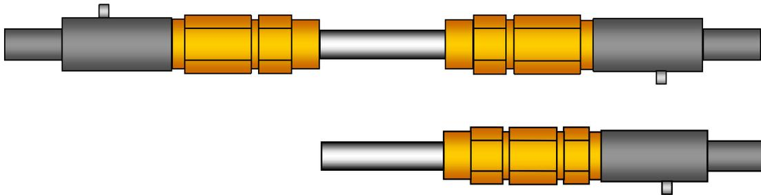
**Figure 4: Test Sample Configurations, Outer Conductor Pull**
