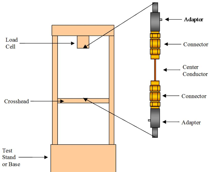
**Figure 2: Diagram of a Typical Test Stand & Device Under Test**
