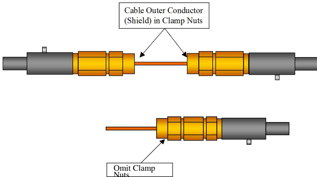
**Figure 3: Test Sample Configurations, Center Conductor Pull**
