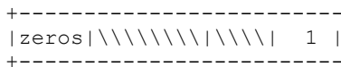
Figure 6.6. The codebook memory, length IMem=85 samples, and the target vector 1, length 22 samples
