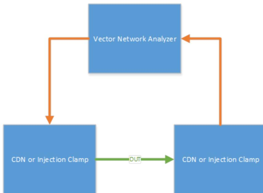
**Figure 1 - Equipment Setup**
